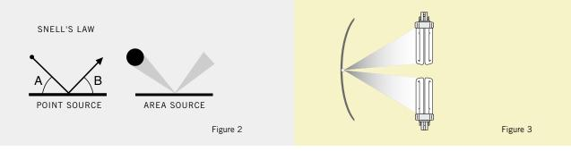
According to Snell's law of reflection, light that is incident upon a specular reflective surface will be reflected at an equal angle. When light is incident throughout a zone, as with compact fluorescent lamps, it is reflected into a zone of equal dimension (Fig. 2).
